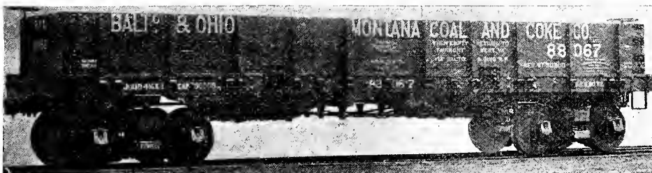
Fig. 26. GONDOLA CAR, WITH TWIN-HOPPERS, FOR COAL. BALTIMORE & OHIO RAILROAD. Length, 36 ft. 2 ins. Capacity, 60,000 lbs. Weight, 30,800 lbs.
